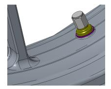
3. Insert Rubber Grommet 2 into Valve body and follow by Washer
