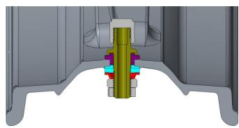
5. Remove Valve Cap and install FOBO Sensor (Please follow FOBO TPMS series installation guide)
