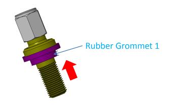
2. With Rubber Grummet 1 at Valve Body, Insert Valve Body into Rim valve hole
