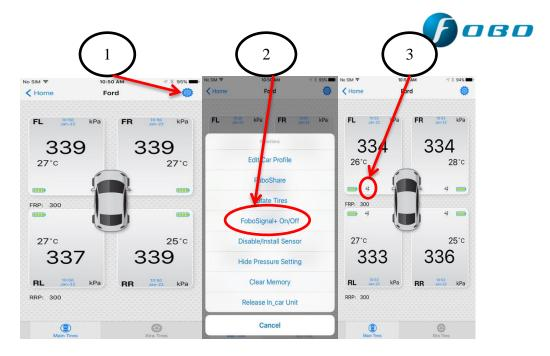
This feature will enhance sensor signal reception. It is useful if the user is facing a problem in receiving signals from the sensors due to interference.
