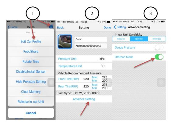
Users can set the Pressure limit below 160Kpa/23Psi if they turn on the Off Road mode.
