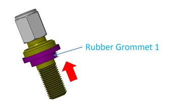
2. With Rubber Grommet 1 at Valve Body, Insert Valve Body into Rim valve hole
