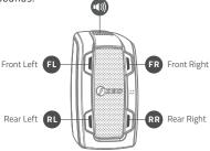
4 x FOBO Tire 2 sensors to measure pressure and temperature in real time. Wirelessly transfer data to in-car unit and smart device.
