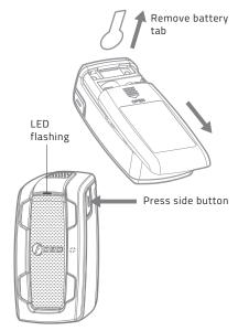
At your vehicle, install one sensor at a time. Unscrew sensor cover FR, remove battery tab, screw back the sensor cover and screw sensor on the tire valve FR. Contnue with sensor RR, RL and finally FL.
